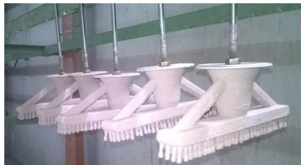
**Gambar 4.12** *Shell Building* saat Proses *Investment Casting*
