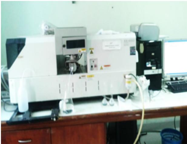
**Gambar 2.** AAS (*Atomic Absorption Spectrophotometric*)
